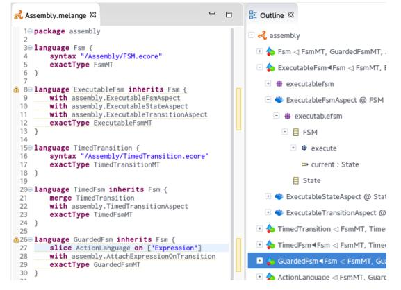
Figure 2: Assembling several variants of a finite-state machine language in Melange. The outline presents the abstract syntax of each language, the methods and runtime data inserted using aspects (*e.g.* a fire() method on transitions and the current state), and the subtyping relations linking their types. Language designers can thus build new languages on the one side and observe the results on the other side at the same time.
