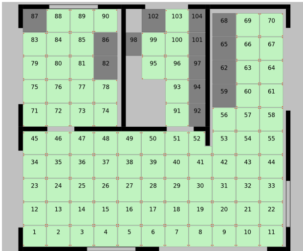
Figure 5: 2D image of the tiles composing the floor, with the sensors highlighted in red. Gray tiles are not equipped with sensors.
