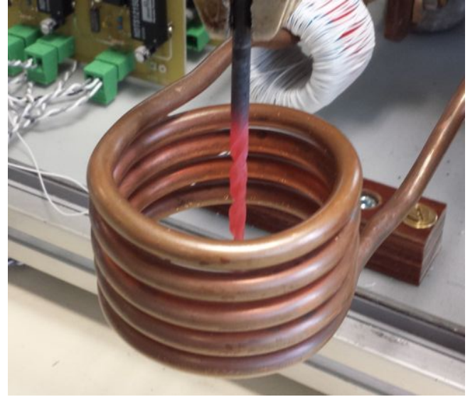
Fig. 4. A heating experiment: Work-piece at around 900^\circ\text{C} .
