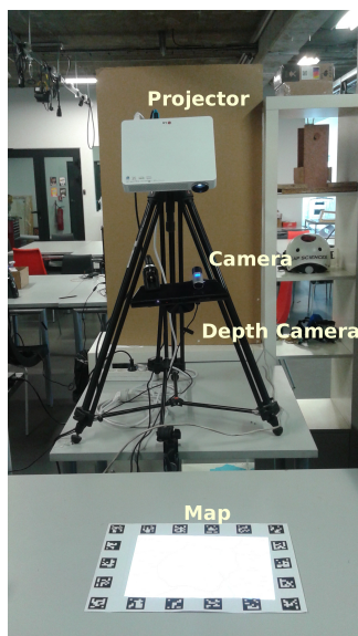
Figure 30: System for the interaction techniques experiment (Museum)
