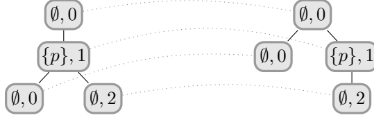
■ Figure 5 Two data trees with \Sigma \stackrel{\text{def}}{=} \{\emptyset, \{p\}\} and \mathbb{D} \stackrel{\text{def}}{=} \mathbb{N} . The bisimulation relation is depicted by dotted grey lines. The left tree satisfies formula (4) at its root, but the right tree does not.
