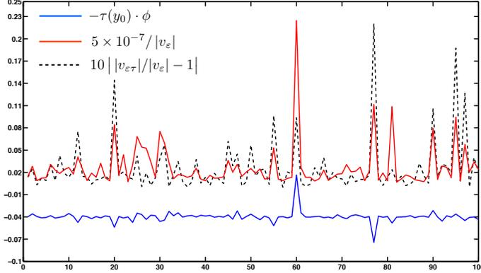
Figure 3: For different random realizations of  $V$ : reconstructed  $\tau(y_0) \cdot \phi$  (the average value is approximately 0.398), amplitude of the measurement without shift and deviation of the ratio  $|v_{\varepsilon\tau}/v_\varepsilon|$  with respect to 1.
