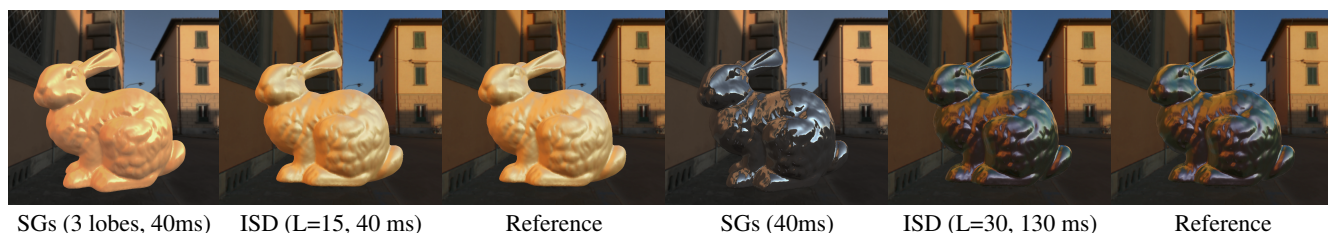
Fig. 8. Qualitative comparison of our technique to shading with Spherical Gaussians, using three lobes [Wang et al. 2009] for the two materials gold-paint and color-changing-paint3 from the MERL database. The lack of stability in the SG fitting process limits the number of basis functions that can be fit, hence reducing the accuracy of the result. At equal speed, our renderings are much closer to ground truth. All SG renderings used in our comparisons have been provided by the authors of [Wang et al. 2009] to match our supplied viewing parameters.
