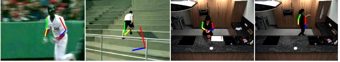
Figure 2: Illustration of human pose estimation used in our experiments [8]. Successful examples and failure cases on JHMDB (left two images) and on MPII Cooking Activities (right two images). Only left and right arms are displayed for clarity.
