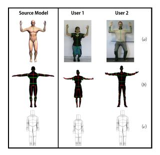
**Figure 4:** Source and user data ((a) and (b)) to find scale values and deform source bounding cage to obtain user-specific cages (c).
