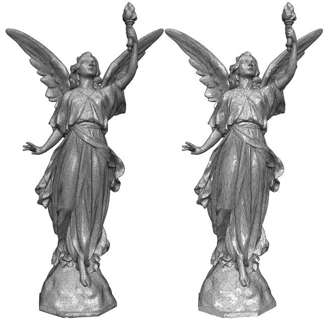
Figure 25: Aggressive simplification. As the tolerance in the Simplification Envelopes is generated by offsetting the vertices along the normals, this approach cannot simplify the geometry of highly undulating surfaces beyond a certain Hausdorff limit. Left: input mesh. Middle: output from the Simplification Envelopes ( H_{|O \rightarrow I} = 60\% ). Right: output from our algorithm ( H_{|O \rightarrow I} = 10\% ).
