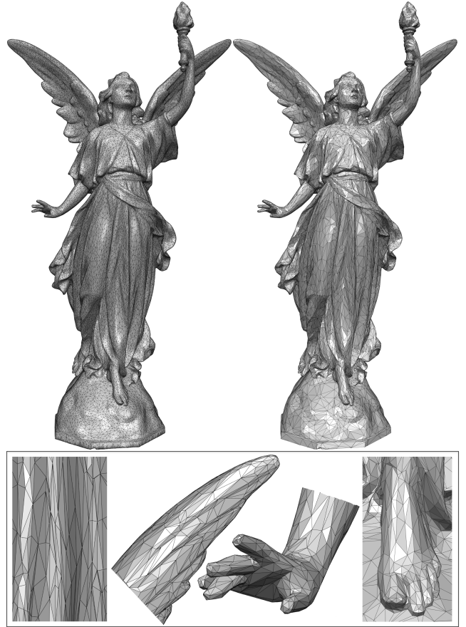
Figure 27: Lucy. Left: Input model (50k). Right: Output from our algorithm (16.7k vertices, \delta = 0.13\% ).
