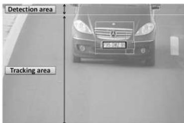
Figure 13: Number plate detection example
