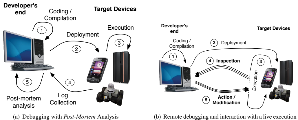
Figure 1 – Log-based Static Debugging vs. Remote Debugging
