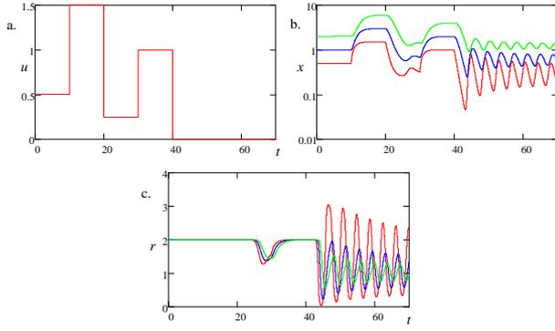
**Fig. 4** The results of simulation for the Goodwin oscillator: (a) input  $u(t)$ ; (b) the state variables  $x_i(t)$ ,  $i = 1, 2, 3$  for the input  $u(t)$ ; (c) the ratio between state variables for  $2u(t)$  and  $u(t)$
