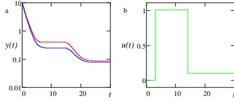
**Fig. 2** The results of simulation for the system (7): (a) output trajectories  $2y_{u(t)}(t)$  and  $y_{2u(t)}(t)$  for the inputs  $u(t)$  and  $2u(t)$ ; (b) input  $u(t)$
