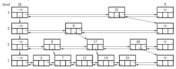
We want to study the length of a path to reach a certain element. For instance, to reach 25, we follow the path 9-17-19-25, and we record 4 steps. A step from the header to the data, as well as steps downwards between header elements are not counted.
