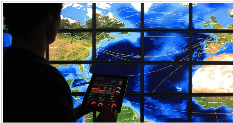
Fig. 19: Interacting with an ultra-wall using a tablet that features both control widgets and an area dedicated to high-precision remote pointing (top-left).
