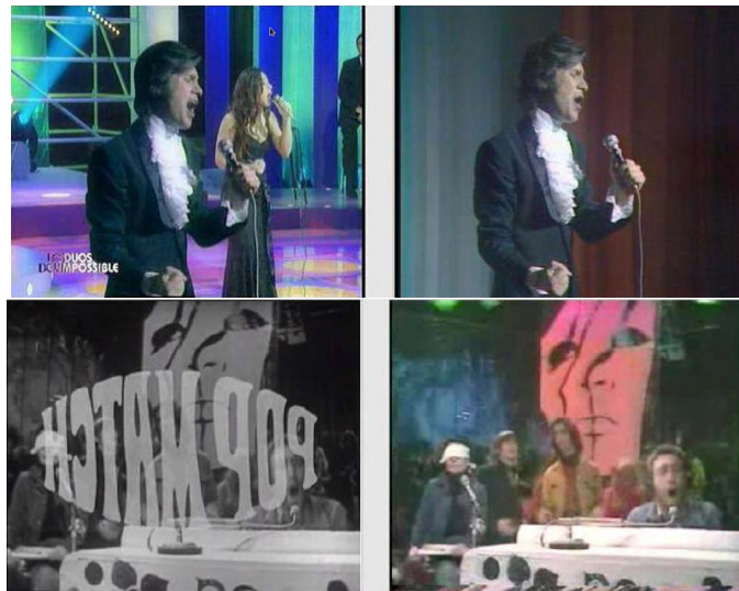
Figure 3.2: Example of two content-based copy detections involving severe alterations between the original video (right) and the broadcasted ones (left)
