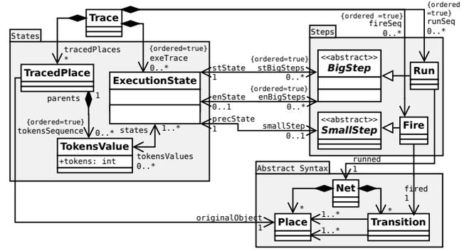
Figure 6: Petri net rich domain-specific trace metamodel
