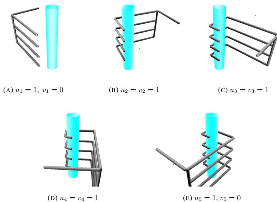
Figure 10: Various stages of the manipulation of a cylinder, whose section is  $\bar{f}_3(O_\omega)$ . Due to numerical and graphical reasons, we extended one more phalanx with respect the configuration described in Theorem 9, so that for every finger the resulting motion control vector is  $u_1 = u_4 = 1, v_1 = v_5 = 0$  and  $u_j = v_j = 1$  with  $j = 2, 3, 4$ .
