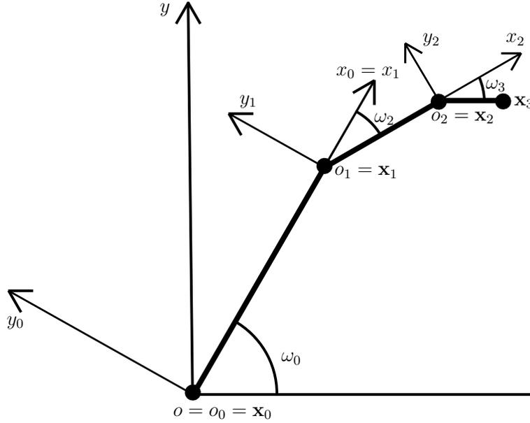
Figure 4: A finger with rotation control vector  $(0, 1, 1)$  (in particular  $\omega_1 = 0$  and  $\omega_2 = \omega_3 = \pi/6$ ) and extension control vector  $(1, 1, 1)$
