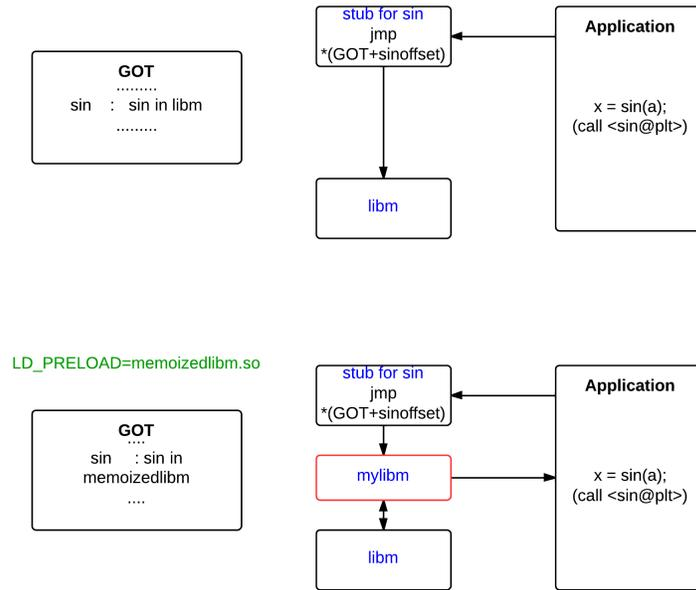
Fig. 2. Intercepting dynamic call to *sin***ALGORITHM 1:** Pseudo code for memoization
