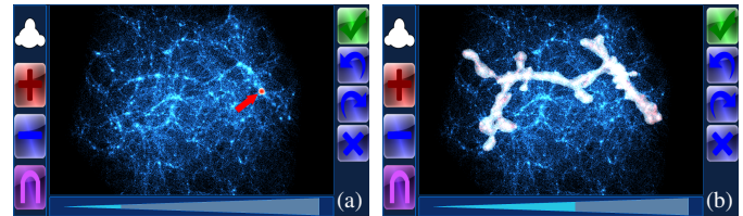
Fig. 14. Uncovering global structures in halos. (a) A small cluster is selected with PointCast. (b) Lowering the threshold reveals structures connecting the initially selected cluster to other clusters in the dataset.
