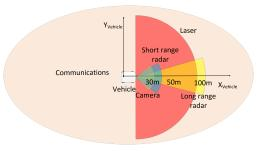
Fig. 1: Field of View of vehicular sensors in comparison with a radio communication range.
