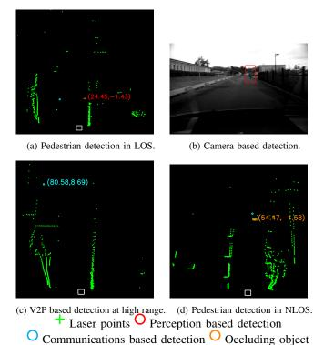
Fig. 3: Obstacle detection in various conditions.
