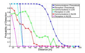
Fig. 4: Detection capabilities of perception and communication in LOS and NLOS conditions.
