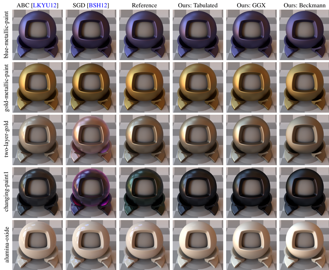
Figure 6: Side-by-side fitting comparisons of a few isotropic materials from the MERL database [MPBM03].
