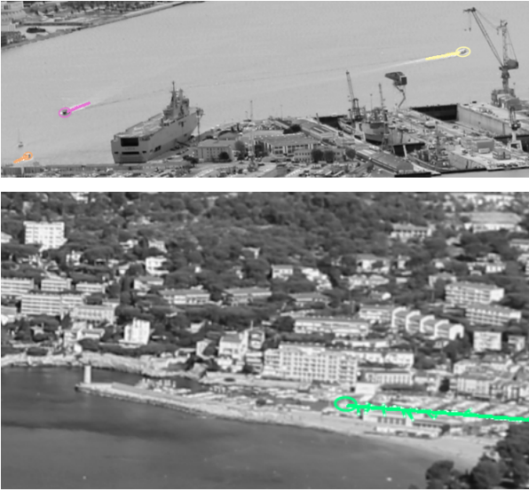
FIGURE 4 – Detection and tracking results on two sequences of simulated satellite images of Toulon. The image sequences are by courtesy of Airbus Defence & Space, France. Top : Tracking results on the first image sequence up to frame 50. Bottom : Tracking results up to frame 150 of the second image sequence.
