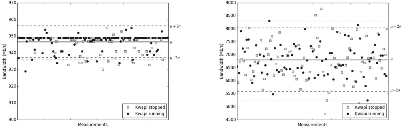
**Figure 6: Measurements of network bandwidth between nodes with/without Kwapi running, for a 1G cluster (left panel) and a 10G cluster (right panel). Solid lines represent the mean  $\mu$  and dashed lines the 2 standard deviations  $\sigma$  from the mean.**
