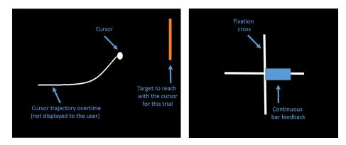
Figure 9: Examples of BCI feedback for BCI based on sensorimotor rhythms. Left: continuous cursor feedback, the cursor continuously moving from left to right, its vertical position being modulated by the sensorimotor rhythms amplitude [7]. Right: bar feedback, a bar is continuously extended towards the left or right, depending on whether the recognised EEG pattern was left or right hand movement, respectively. The bar length is proportional to the absolute classifier output [37].
