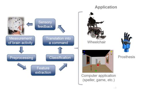
Figure 1: General architecture of an online brain-computer interface, with examples of applications.
