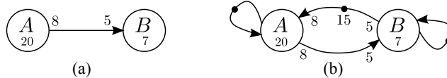
Figure 2: (a) An SDF graph; (b) The same graph with channel size constraint and auto-concurrency disabled.
