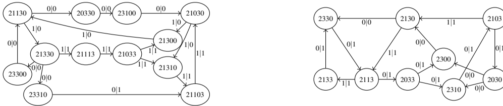
(b) \mathcal{T}_B corresponds to \mathcal{T}_A when unused transitions are deleted.
