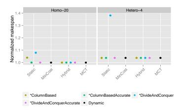
Figure 4. Makespan for different algorithms for HOMOGENEOUS-20-CPUS and HETEROGENEOUS-4-GPUS for static setting.
