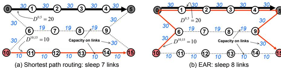
Figure 1: Example of shortest path routing and EAR.
