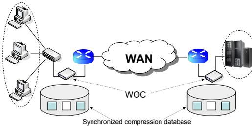
Figure 2: Reduction of end-to-end link load using WOC
