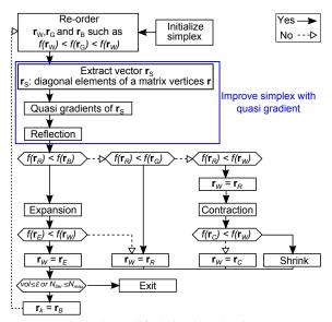
Figure 4: Modified Simplex Algorithm.
