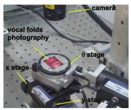
Figure 9: Photography of the microrobotic cell.
