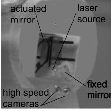
Figure 14: Photography of the developed endoscopy tip.
