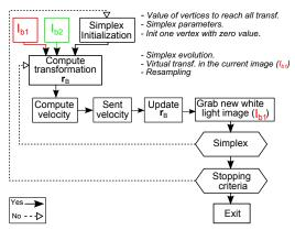
Figure 6: MI-based visual servoing scheme.
