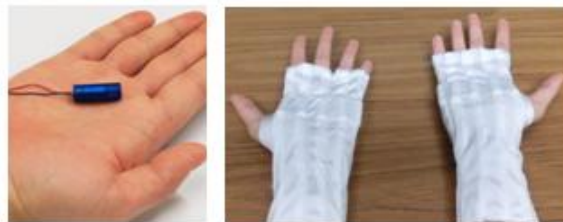
Fig. 4. Left: A vibration motor. Right: Our gloves with 10 embedded motors (5 per hand). In the tactile feedback condition, individual motors are activated to represent the classifier output.
