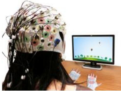
Fig. 1. A participant receives tactile feedback while controlling the MI-BCI. Vibrations from the motor on the right hand represent the current feedback provided by the MI-BCI system.
