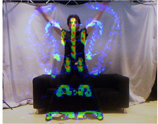
Fig. 4: The histogram heat map during the jumping jack exercise. Red spots highlight the start/stop position of each body articulation.
