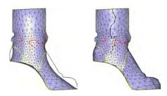
Fig. 9. Silhouette matching: Projection of most protruding edges to the silhouette and mesh deformation best preserving normals. The silhouettes strokes of the side-view are perfectly matched, as well as the 3D feature line constraints (yellow). The mesh edges marked in black on the bootleg are the selected edges tied to the silhouette stroke of the front view.
