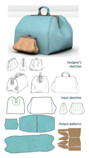
Fig. 15. Top: Doctor bag and leather purse designed with our system. Middle: designer's sketches exhibiting design folds which are indended to remain permanently on the product and the sketches given as input to our system. Bottom: the patterns we output. Note that we did not use symmetry for these examples: therefore, neither the input sketches nor the resulting shapes or patterns are fully symmetric.
