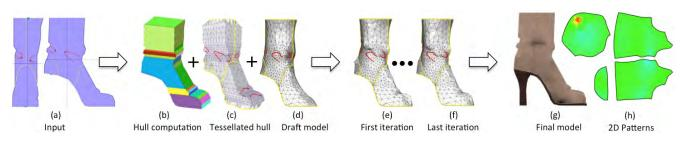
Fig. 3. Processing pipeline: Input (a); Initialization (b,c,d); Iterative optimization (e)...(f); Results (g,h).
