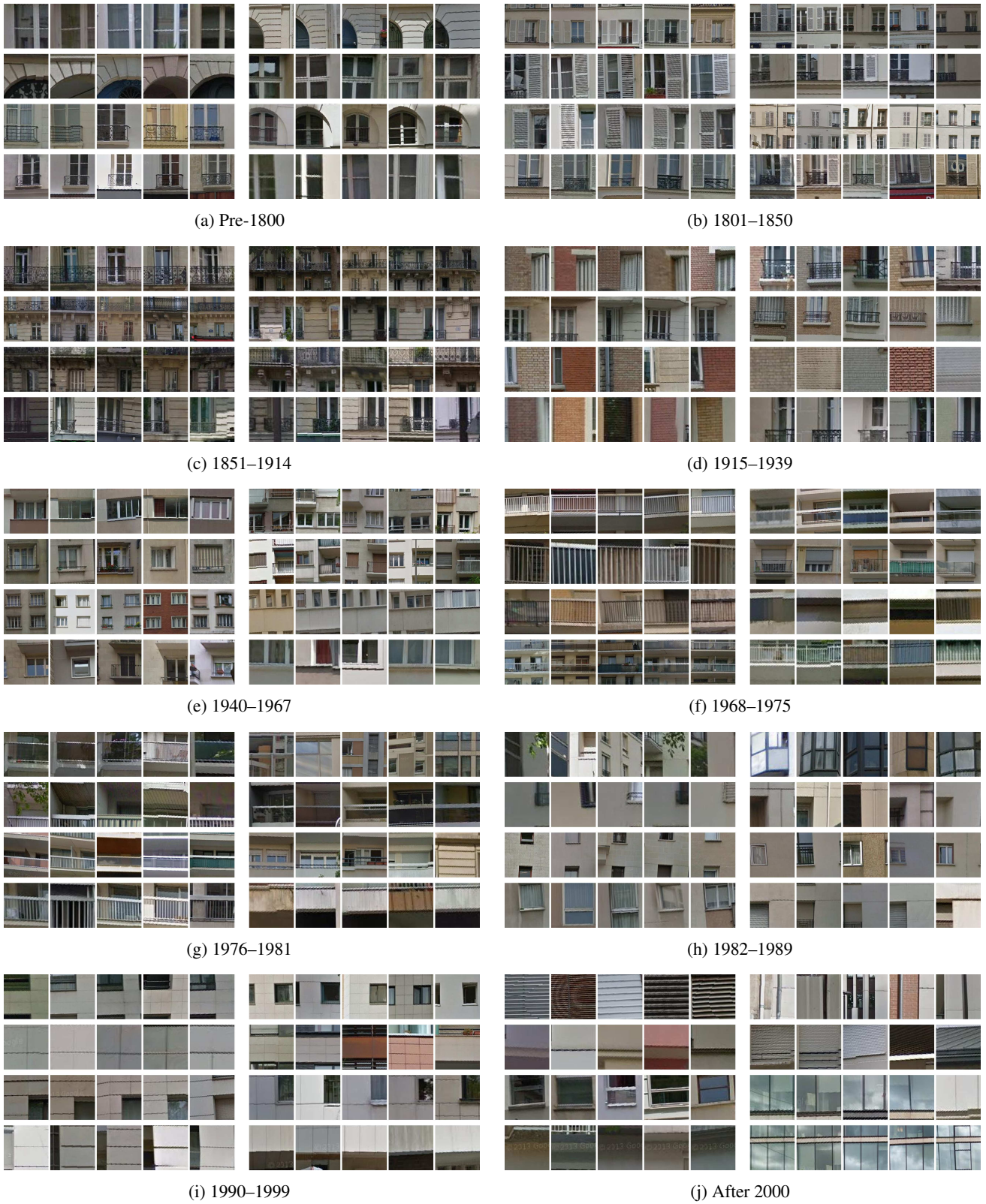
Figure 4: Top 8 discriminative elements for each period. For each element, five example patches are shown in a row. Notice how as we move towards modern times the patches largely become repeated geometries.
