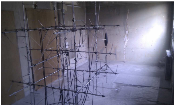
Fig. 2. Pictures of the experimental microphone array. The 120 electret microphones are at the ends of the small rods, randomly placed and oriented on 15 fixed bars. The microphones are omnidirectional in the used bandwidth.
