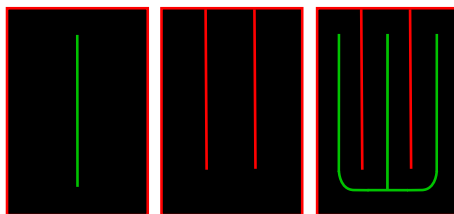
Fig. 3. At the left, the skeleton (in green) extracted with Cornea’s original method. A spatial partition can be generated (red lines) to constraint skeleton computation to a more branched shape. At the right, the skeleton computed by Cornea’s method when all red points are considered as contour points.
