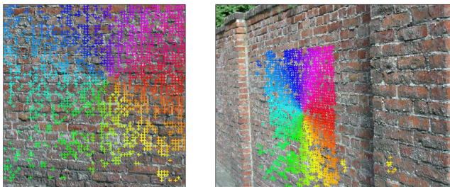
Fig. 8 Matching result between two images with repetitive textures. Nearly all output correspondences are correct. Wrong matches are due to occluded areas (bottom-right of the first image) or situations where the deformation tolerance of DeepMatching is exceeded (bottom-left of the first image).
