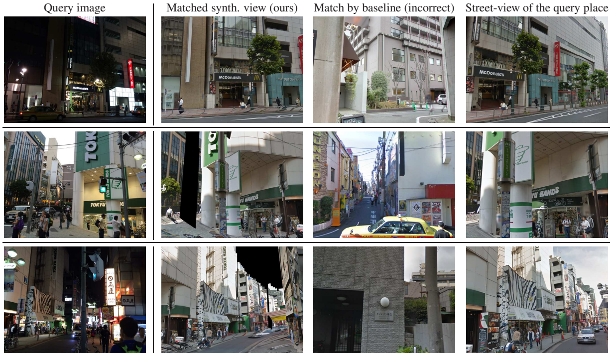
Figure 9. Example place recognition results with synthesized views (our method) compared to using only the original Google street-view images. (Left) Query image. Note the difficult illumination. (2nd column) The best matching image (correct) by our method (Dense VLAD descriptor with the database expanded by synthesized views). (3rd column) The best matching image (incorrect) by Dense VLAD matching but using only the original street-view images. (4th column) The original street-view database image at the closest position to the query. Our method (2nd column) that uses virtual views with very similar viewpoints to the query can localize queries with difficult (night) illumination, thus enabling true 24/7 localization. This is not possible using the original street-view images (last column), which depict the same places but from quite different viewpoints. Please see additional results on the project webpage [16]
