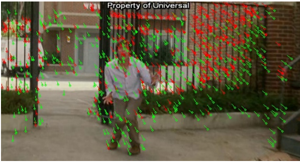
Fig. 2 Visualization of inlier matches of the estimated homography. Green arrows correspond to SURF descriptor matches, and red ones are from dense optical flow.
