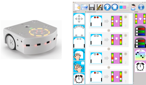
Fig. 1. The Thymio II robot (left) and a screenshot of the VPL programming environment for children (right).
