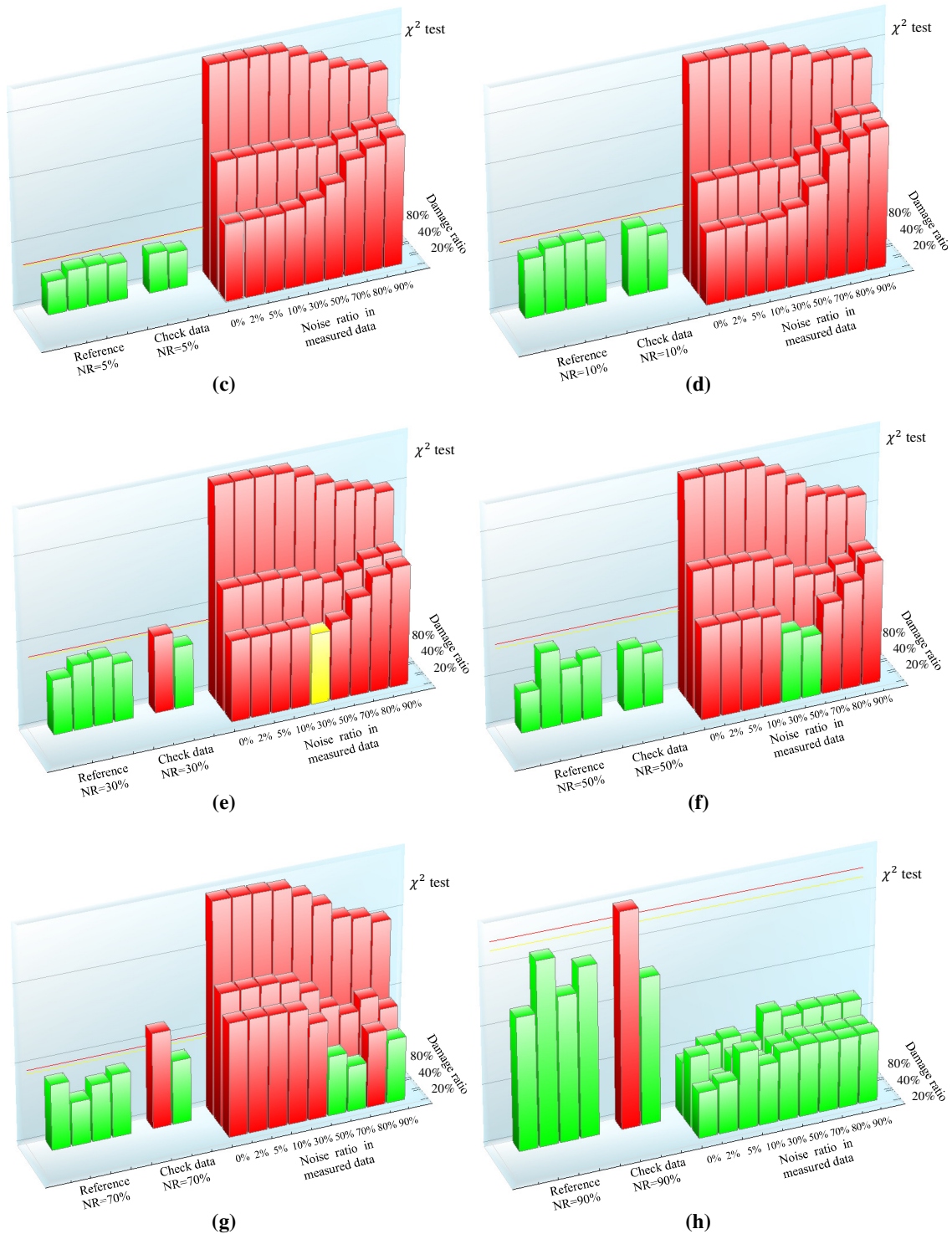
Figure 7. \chi^2 test from SSDD technique for different damage and noise ratios in reference and checking data: a with no noise in reference data, b noise ratio of 2%, c noise ratio of 5%, d noise ratio of 10%, e noise ratio of 30%, f noise ratio of 50%, g noise ratio of 70% and h noise ratio of 90% (green: safe zone, yellow: critical zone and red: unsafe zone)
