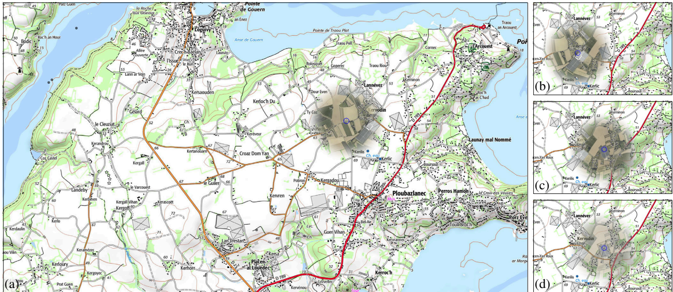
Figure 6. Technique BL: When the two images are overlaid in the same viewport, the lower layer can be revealed in a locally-bounded region only – instead of the entire viewport – using a Blending Lens. The lens punches a hole through the upper layer, revealing the lower layer. (a) & (b) The lens approaches from the left the same facility F as in previous figures. (c) The lens is centered above it, revealing its appearance in the orthoimagery. (d) The lens' transparency can be adjusted using alpha blending, so that both images are visible simultaneously, as with the overlay technique (OV).
