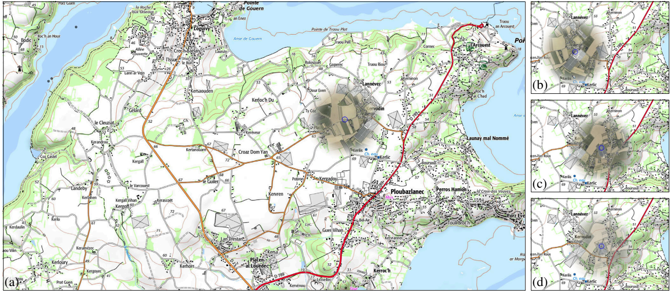
Figure 6. Technique BL: When the two images are overlaid in the same viewport, the lower layer can be revealed in a locally-bounded region only – instead of the entire viewport – using a Blending Lens. The lens punches a hole through the upper layer, revealing the lower layer. (a) & (b) The lens approaches from the left the same facility F as in previous figures. (c) The lens is centered above it, revealing its appearance in the orthoimagery. (d) The lens' translucency can be adjusted using alpha blending, so that both images are visible simultaneously, as with the overlay technique (OV).
