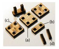
**Figure 6:** The wooden pieces of the last prototype: (a) central support, (b) rod guides, (c) encoded caps, (d) assembling bars.
