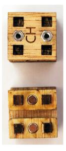
**Figure 7:** Extension to the last prototype: magnets make it possible to change dominos' encodings.
