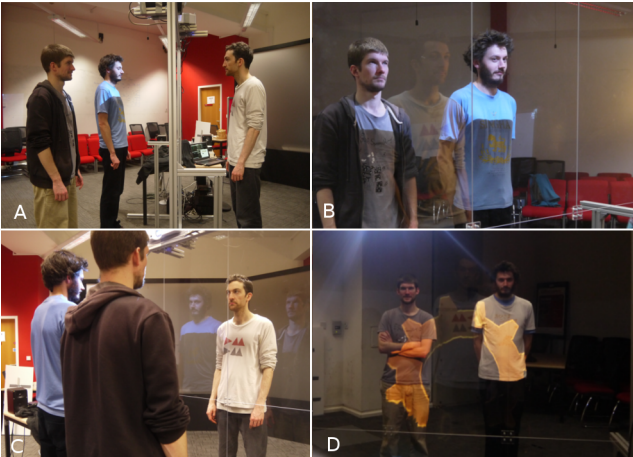
Figure 3: A) Shared space created by the optical combiner. B) and C) The three users can all be perceived from both sides. D) Virtual content (here a cog) can be revealed from both sides and appears in the shared space at the correct depth for all users.
