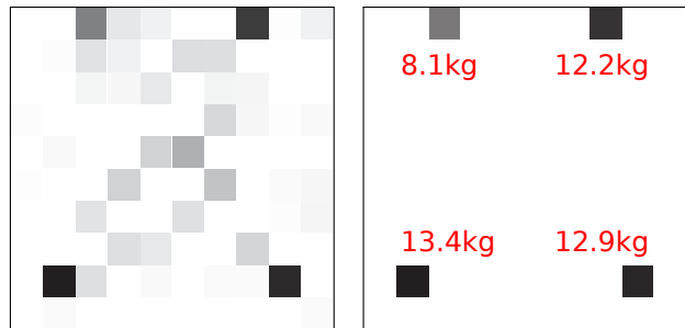
(c) The pressure scan obtained without noise filtering. Most of the noise is caused by sensor noise. The highest pressure is encoded as black.
