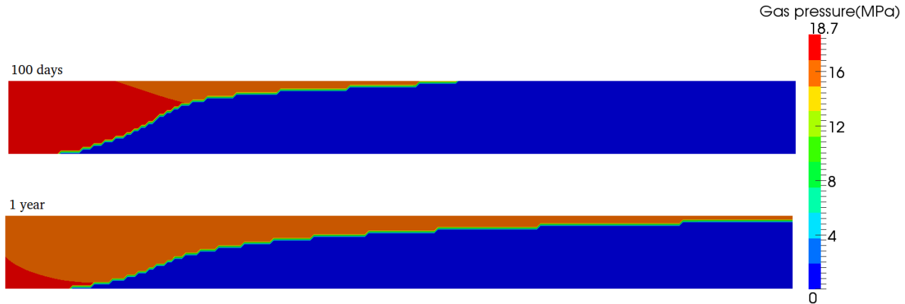
FIGURE 4. Gas pressure P_g after 100 days and 1 year of \text{CO}_2 injection. Only the 1.1 km closest to the injection is presented.
