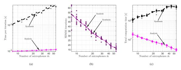
Figure 2. Computational cost *vs* number of microphones m̃. (a) Time per LSMR iteration. (b) Number of SDMM iterations. (c) Total computation time.
