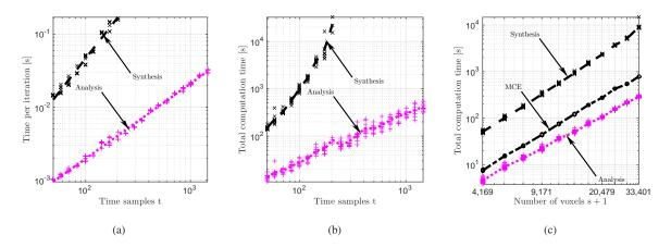
Figure 1. Computation time relative to the problem size. (a) Time per LSMR iteration vs t (wave equation). (b) Total computation time vs t (wave equation). (c) Total computation time vs s + 1 (Poisson's equation).
