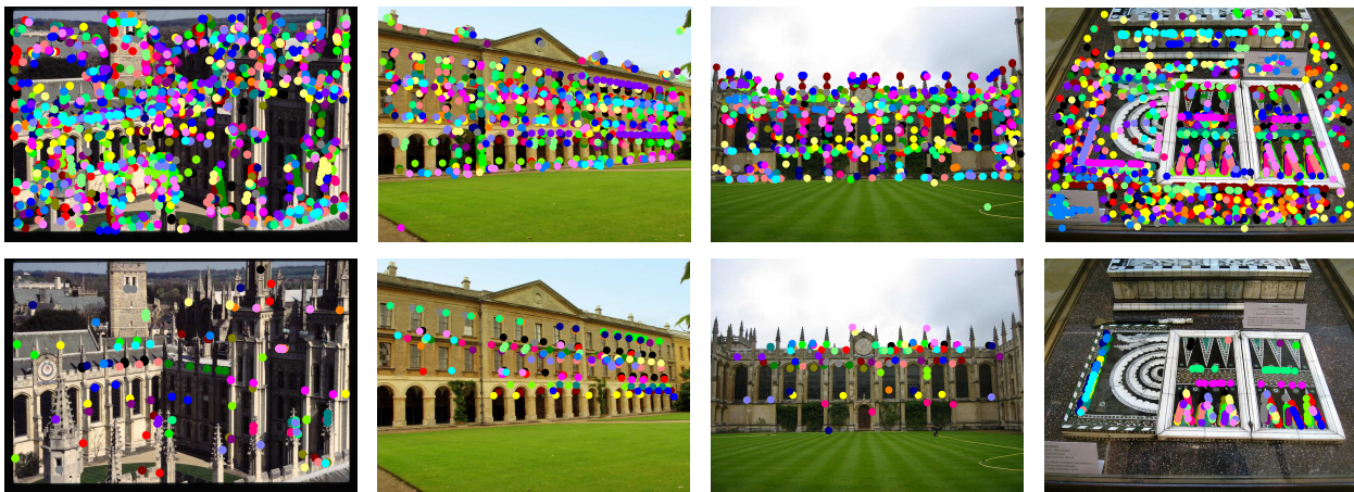
Fig. 2 Examples of features mapped to the same visual word, finally being aggregated. Examples shown for a small codebook of 128 visual words (top), which is a typical size for VLAD, and a large one of size 65k (bottom), which is a typical size for ASMK. Each visual word is drawn with a different color. Top 25 visual words are drawn, based on the number of features mapped to them.
