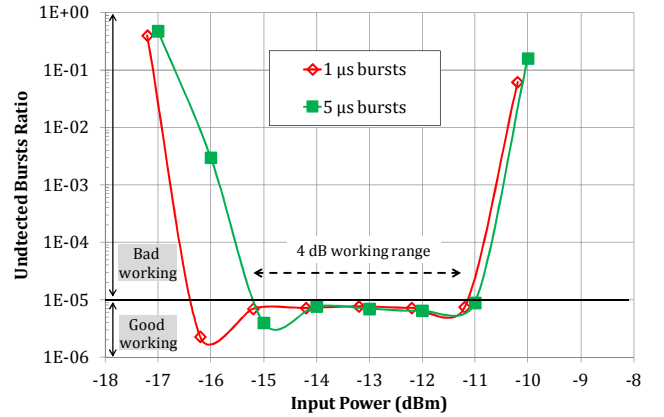
Fig. 6. Undetected bursts ratio versus optical input power ( P_i ) in the label extractor for I_{SOA} = 45 mA.
